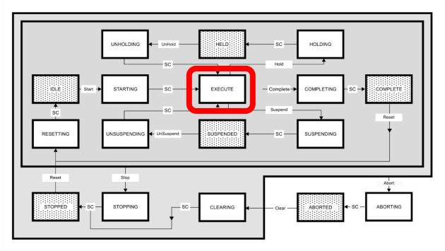
$Performance = \frac{Total\ Quantity\ Produced\ at\ this\ machine}{Time\ machine\ is\ producing\ Product(Execute)\ *\ Maximum\ Machine\ Speed}$
