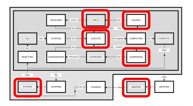
$Availablity = \frac{Time \ machine \ is \ Producing \ Product \ (Execute + Holding + Suspending)}{Time \ machine \ is \ producing \ Product + Time \ when}$  $machine \ is \ in \ faliure \ (Held \ Stopped \ Aborted)$
